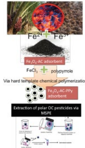
Figure 2: Synthesis of \text{Fe}_3\text{O}_4 -POAC and \text{Fe}_3\text{O}_4 -POAC-PPy adsorbents and the extraction using MSPE method.
